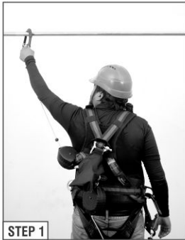
STEP 1 Connect one leg of the SRL to a pre-checked anchorage point and secure lock with the help of the hook.
