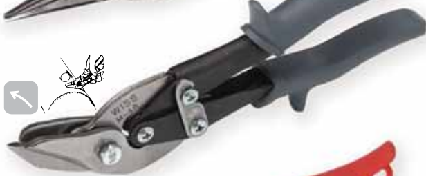
M4R Pipe & Duct Snip • For metal pipe and duct • Double-cut design curls 11/64" strip of metal safely away, leaving two clean, straight edges
