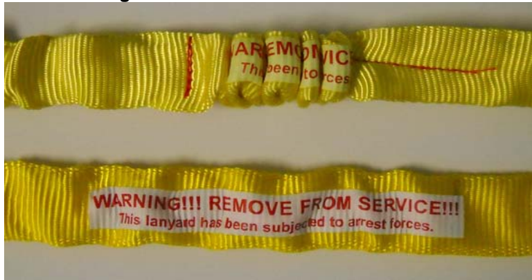
Fig 10.1 – Internal SAL Indicator Label
