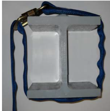
Incorrect Tie-Back Connection
