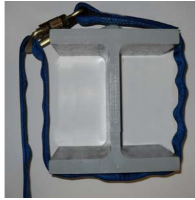
Incorrect Tie-Back Connection
