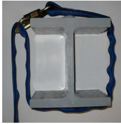
Incorrect Tie-Back Connection
