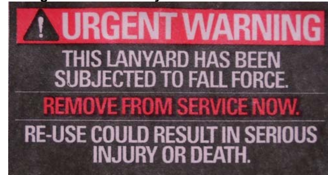
Fig. 10.2 – "Pack-Style" SAL Indicator Label
