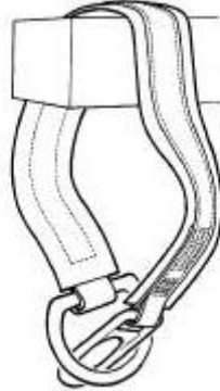
Fig. 3.4 Correct Installation of Web Pass-Thru Sling Anchor
