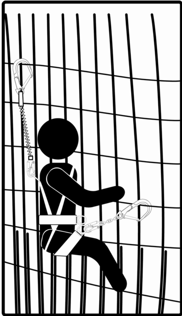
Fig.3.4 Typical Use of Tower Seat Sling
