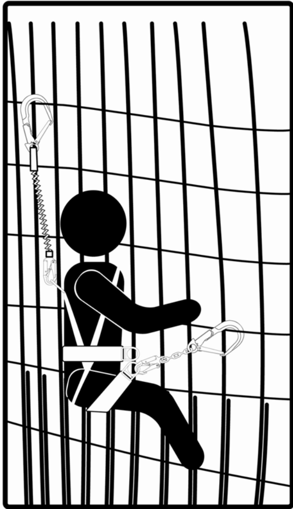
Fig.3.4 Typical Use of Tower Seat Sling
