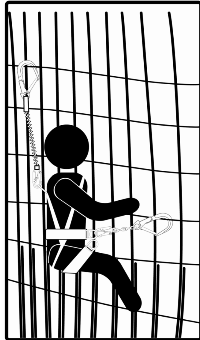
Fig. 3.3 Typical Work Positioning
